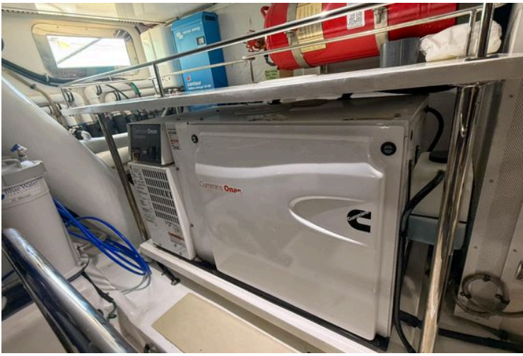
Engine room of 2018 Marlow 53E yacht with Cummins Onan generator and safety equipment.
