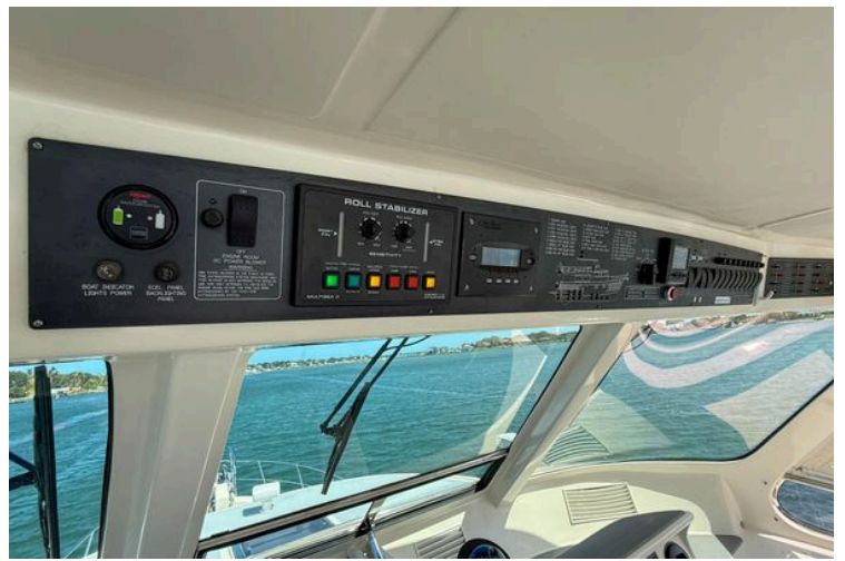
Control panel of a 2018 Marlow 53E yacht with roll stabilizer system.
