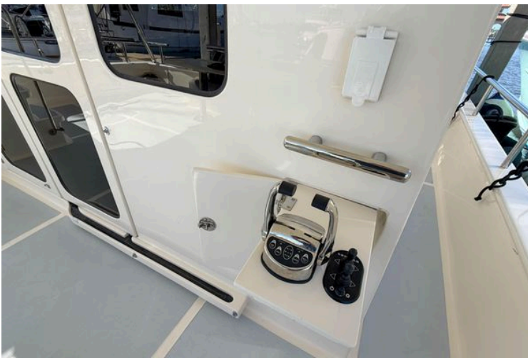
Control panel on 2018 Marlow 53E yacht deck, featuring throttle and joystick controls.
