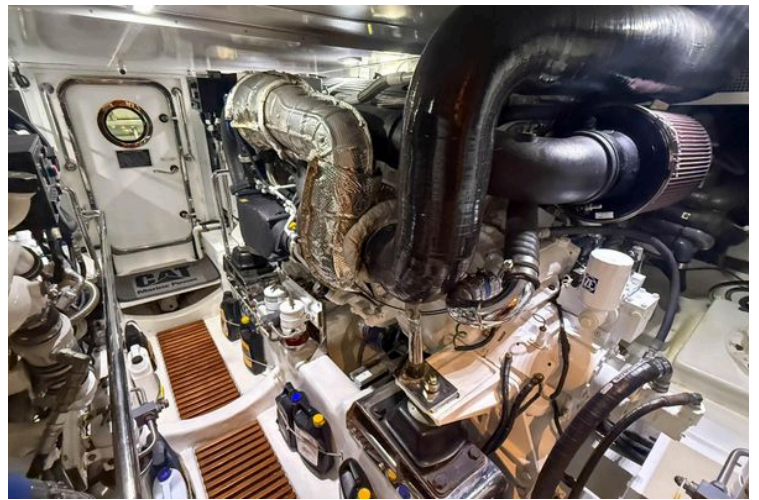
Engine room of a 2018 Marlow 53E yacht, featuring CAT Marine Power components.
