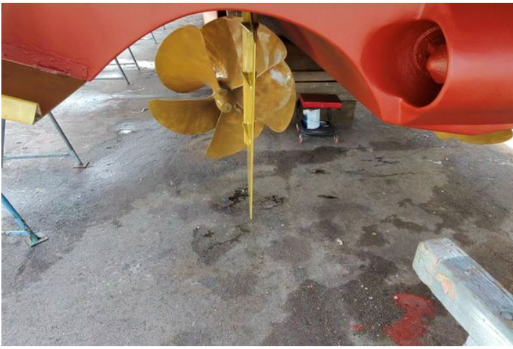
Propeller of 2018 Marlow 75E-CB yacht on dry dock, showcasing bronze blades.
