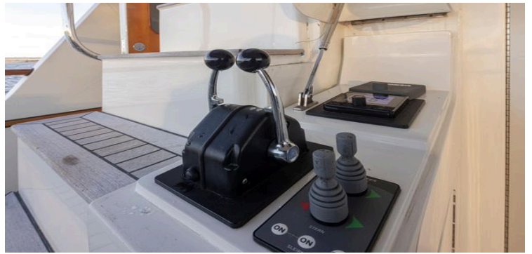
Control panel of a 2003 Marlow 72C yacht with throttle levers and joystick controls.
