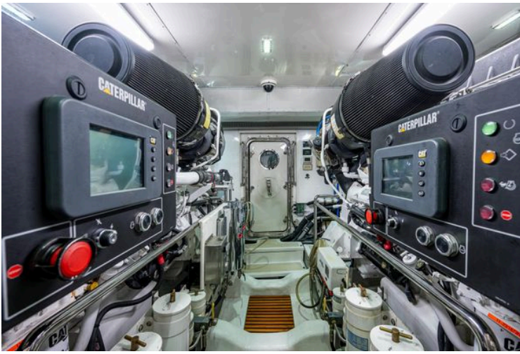
Engine room of a 2013 Marlow Explorer Enclosed Bridge (CB) yacht with Caterpillar engines.
